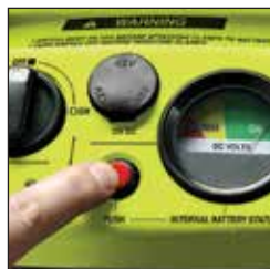
Internal battery status gauge.
