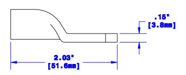
Property of 1-2 [40-32mm<sup>2</sup>] QUICKCABLE Magna Lug W/ Sight Hole 3700 Quick Drive Franksville, WI 53126 U.S.A. 8801F www.quickcable.com Confidential and Proprietary Information Drawing # Material & Treatment C 8801F-INFO **Copper Tube** Tin Plated Shoot 1 er 1
