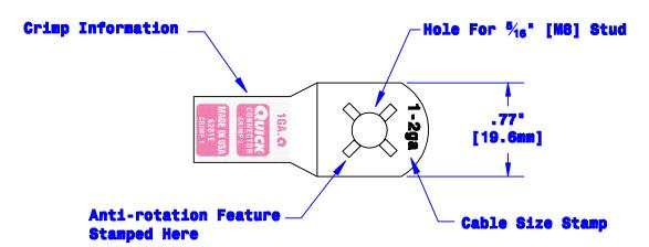
ID Sized For 1-2ga. [40-32mm²] Stranded Cable ¾" [19.1mm] Min Depth
