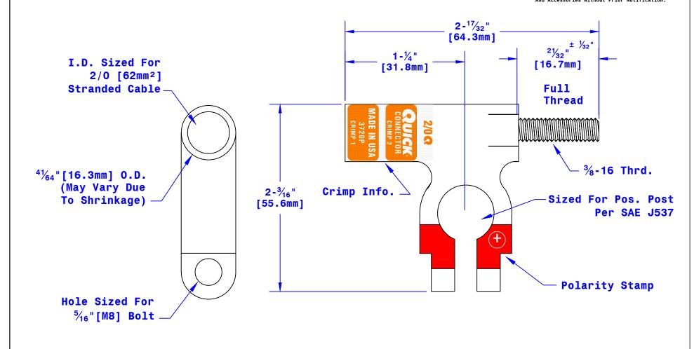
NOTE: Max Torque = 170 In.-Lbs [19.2Nm]
