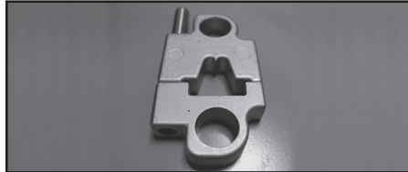
Assemble die set with vertical pin lubricated with Molybdenum grease.
