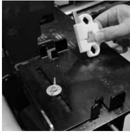
8. Assemble B-crimp die set; pull release handle.
