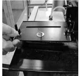
3. Select and install B-Crimp guide plate.
