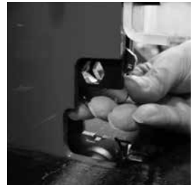
3. Install other die in upper position.
