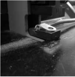
Correct placement of braze seam flag connector in lower die.
