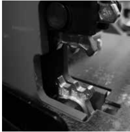
2. Be sure to install the dies so the pockets are matched.
