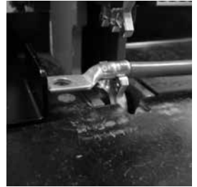
3. In this case the connector is crimped in the near side die pockets.
