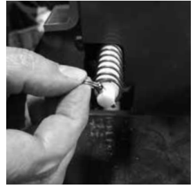
6. Remove retaining pin and spring from upper die pin.
