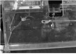
6. Lower shield and connect air supply. Press foot switch to crimp connector.
