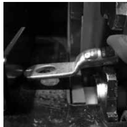
5. Adjust guide plate so that connector is positioned in die set for 1st crimp.
