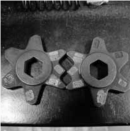
1. These are Diamond Crimp dies. Note that one side has 2 pockets, and so these must be matched.
