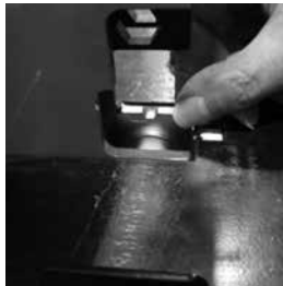
2. Install one die in lower position.
