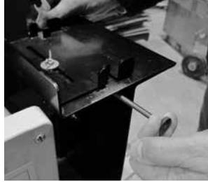
Spring loaded lower die retainer.
