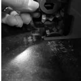
2. Installing Diamond Crimp dies, maintaining the matching pockets.
